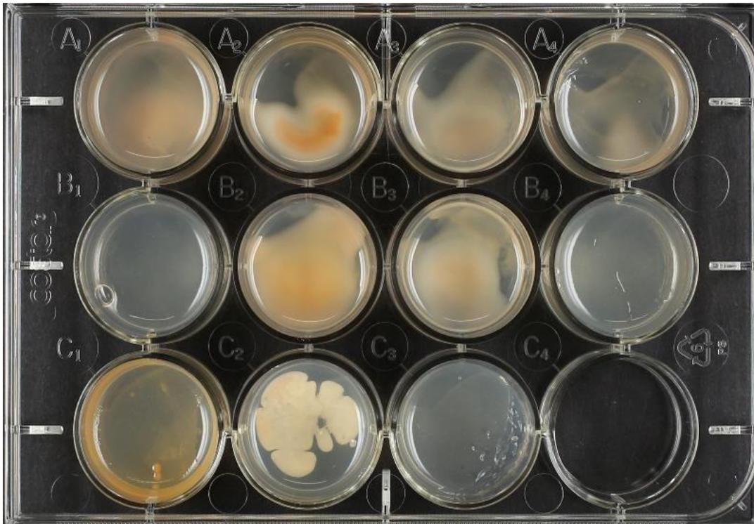
**Sodium chloride tolerance test (from top left to bottom right: 0%, 2,5%, 5%, 7,5%, 10%)**
