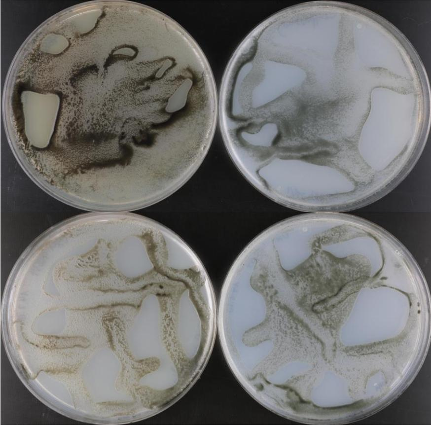
**Carbon utilization test (from top left to bottom right: glucose, arabinose, sucrose, xylose, inositol, mannose, fructose, rhamnose, raffinose, cellulose)**
